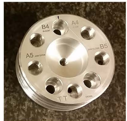
Motor end cover used as manifold for the Jaw cylinder (item 13)
